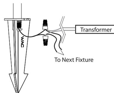
Note: To install multiple fixtures, also connect the power supply wire of each additional fixture to the connection described in 7 of the previous fixture.
