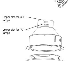
Drop lens trim twists clockwise to install
