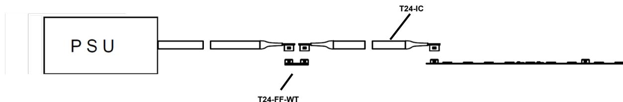
To extend the cable length between power supply cable or a wiring box to a tape sections, (if needed), In Wall Rated Extension Cable (T24-EX3) can be used to join between sections by soldering as shown below:
