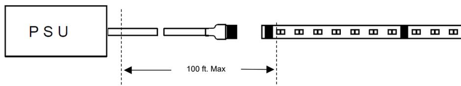
To extend the cable length (if needed), In Wall Rated Joiner Cable (T24-IC) and Joiner Cable Extender (T24-FF-WT) can be used to join between sections as shown below:
