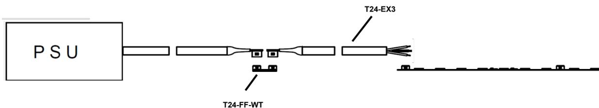
3. Connect electrical power feed connector to any connector on the tape or accessories. There is no polarity. Power feed and connectivity can be done with all directions.
